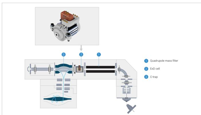
**Figure 1.** Schematic of the ExD cell in the Thermo Scientific Q Exactive Orbitrap mass spectrometer.
